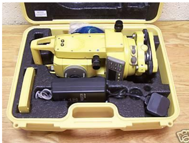
Electronic Theodolite (Topcon DT-200)
