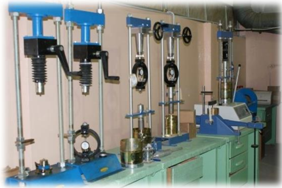
California Bearing Test Device
